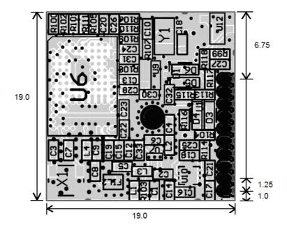
Figure 1: PCB Board dimensions (mm)
